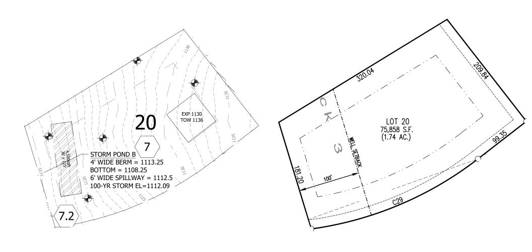
Grading Plan N.T.S Plat N.T.S
